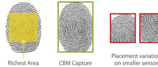
The CBM's capture surface (14x22mm) ensures that the richest area on fingerprints is systematically captured time after time. Acquisition surface contributes significantly to the overall biometric performance:
