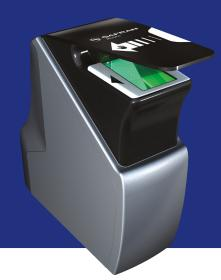
Morpho*Wave*<sup>™</sup> Desktop is a contactless fingerprint acquisition solution. This innovative device captures four finger images with a single movement in less than a second. Its dynamic acquisition capability allows subjects to be 'on the move' during fingerprint capture. Morpho*Wave*<sup>™</sup> Desktop is well suited for high traffic environments.
